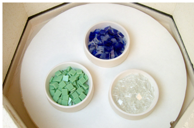
Place the filled casting molds in the kiln
