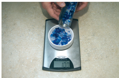
Use a digital scale to fill the casting mold
