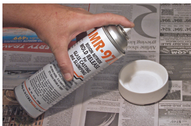
Prepare the C105 using mold release
