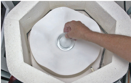
Place the pre-cast foot disk into the reservoir
