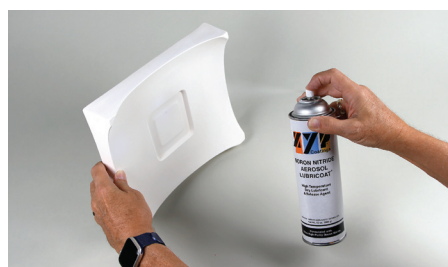
Coat the C225 mold with ZYP™ Boron Nitride
