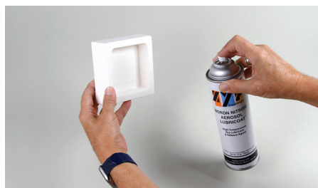
Spray ZYP™ Mold Release on the C110 mold
