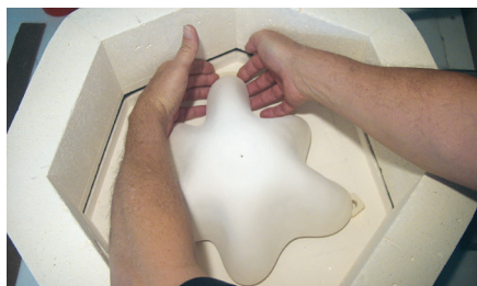
Place the mold in the kiln resting on 3 kiln risers
