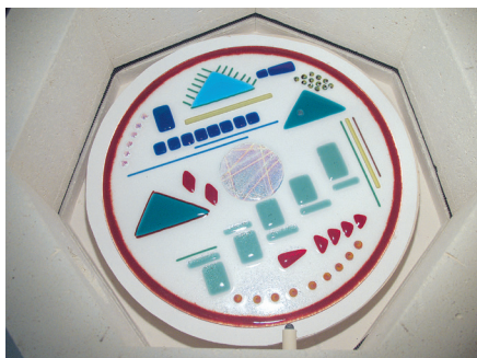
Flat glass disk still in the kiln after fuse firing
