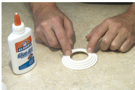
Creating the tapered cone foot assembly
