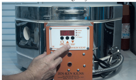
Program the digital kiln controller
