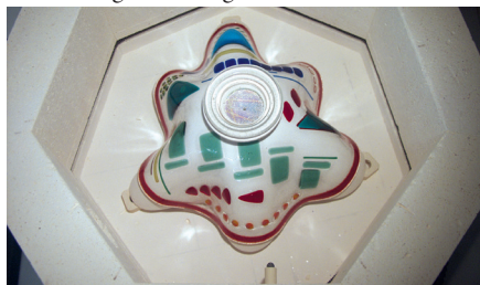
The finished bowl in the kiln after mold forming
