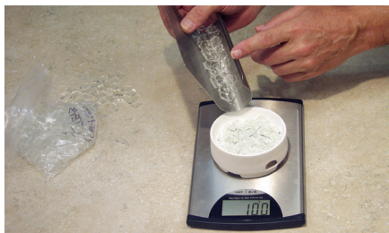
Filling the casting mold using a digital scale
