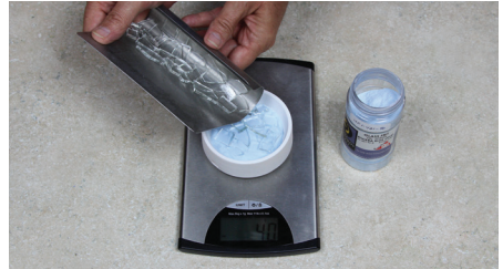
Filling the C100 casting mold using a digital scale
