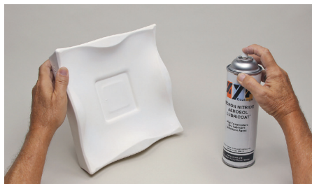
Coat the C220 mold with ZYP™ Boron Nitride
