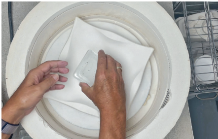
Place the pre-cast square foot into the reservoir
